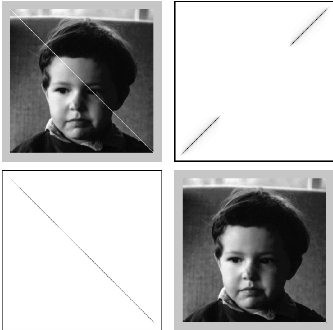
Figure 5: Top left: positive boy figure with diagonal line. Top right: framed negative filtered Fourier transform of top left figure. Bottom left: framed negative frame expansion of the inverse Fourier transform of top right figure. Bottom right: positive restored boy figure.
