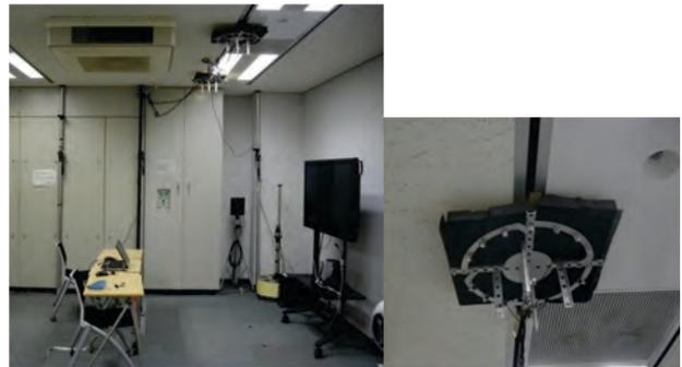
Fig. 4 The microphone arrays attached in the ceiling.
