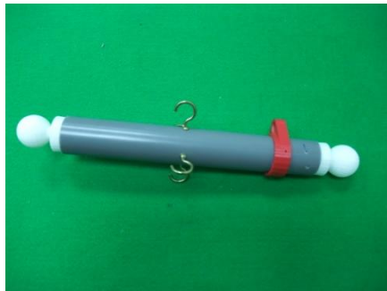
Fig. 6. The basic leg bone represents the simplified leg of Nao.
