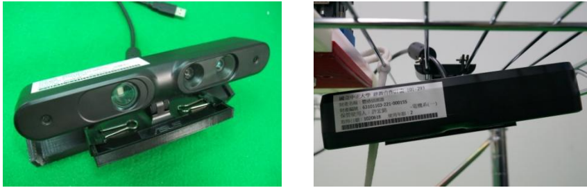
Fig. 3. Asus Xtion Pro Live RGB-D device and suspend on the top the frame.
