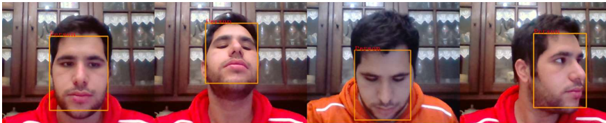
Fig. 7. MTCNN detecting user with different face poses, facing different directions.
