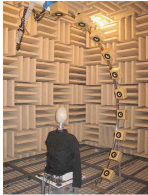
Fig. 7. Photograph of the setup for sound localization experiments. TeleHead with simplified dummy head is set in the anechoic room. Loudspeakers are set in the median plane from -45 deg to 75 deg at intervals of 15 degrees 1.2 m in front of TeleHead.
