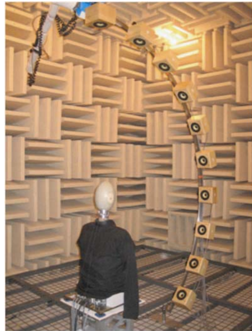
Fig. 7. Photograph of the setup for sound localization experiments. TeleHead with simplified dummy head is set in the anechoic room. Loudspeakers are set in the median plane from -45 deg to 75 deg at intervals of 15 degrees 1.2 m in front of TeleHead.
